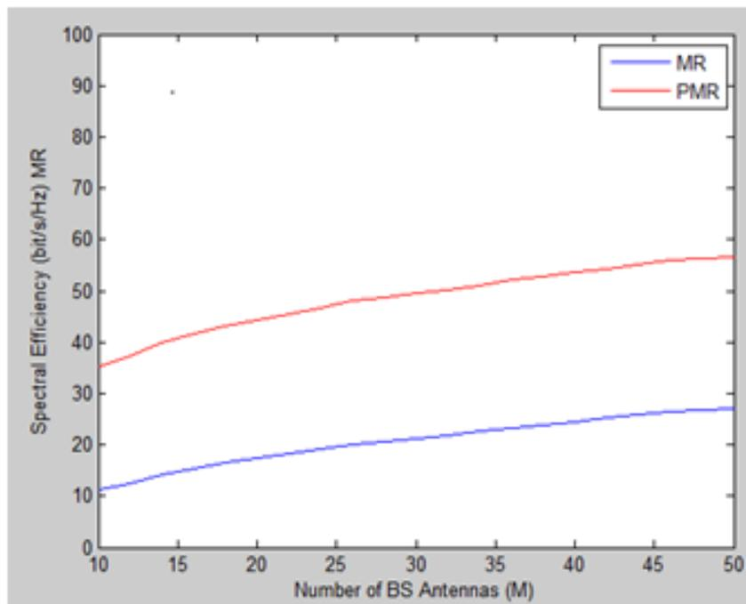
Fig. 4: Simulation with MR Precoding
