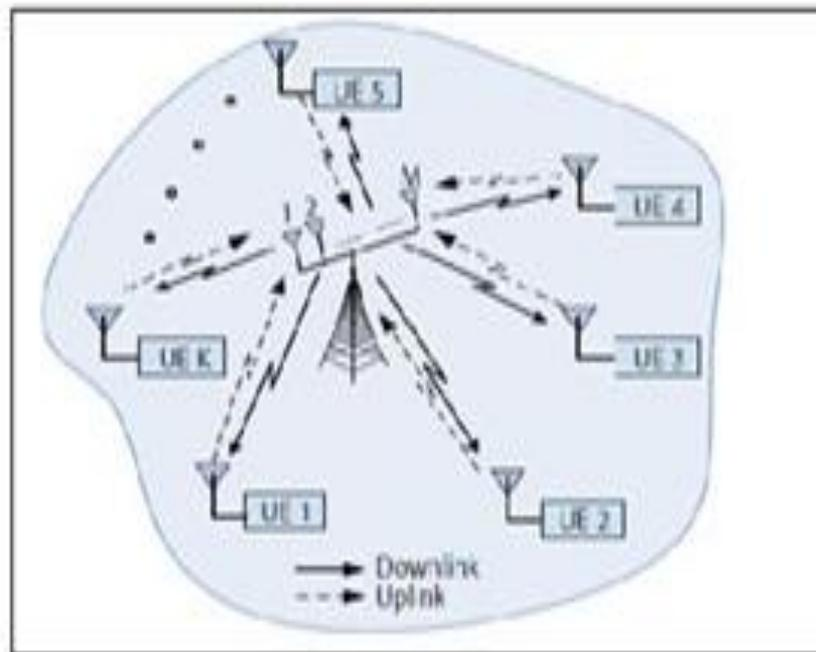
Fig. 2: Hyper- MIMO: a multi-user MIMO technology [7]
